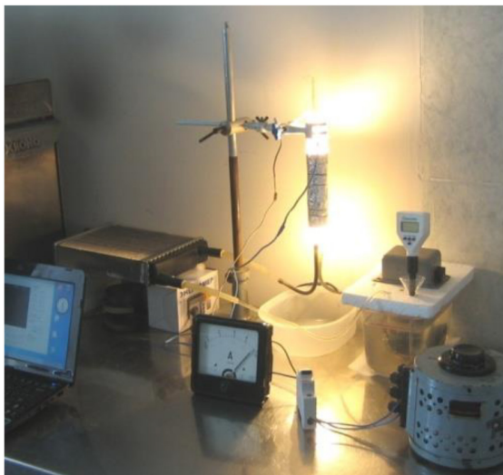
Figure 12. Experimental setup with a circulating \text{KNO}_3 solution and a halogen incandescent lamp.
