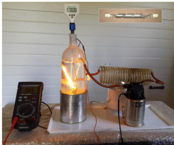
Figure 13. Halogen incandescent lamp wrapped with a tin-lead alloy tape in a vessel with water. The water is pumped through a fan-cooled coil.
