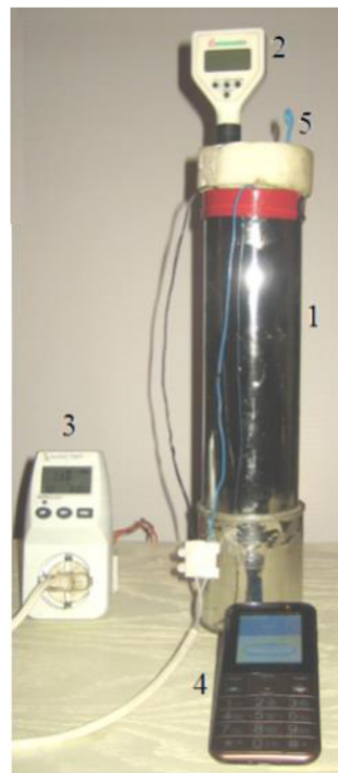
Figure 5. Water calorimeter. 1 – Dewar vessel with water in which an incandescent lamp is immersed, 2 – thermometer, 3 – meter of current, voltage and power consumption, 4 – stopwatch, 5 – stirrer.
