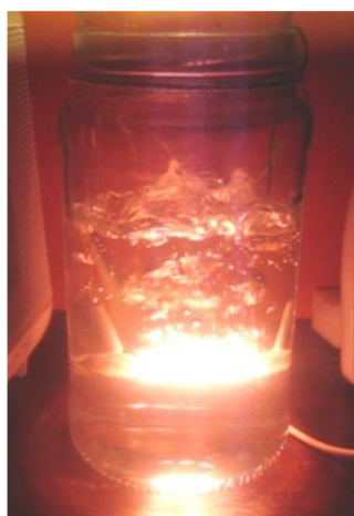
Figure 14. Halogen incandescent lamp in boiling water with \text{NaBiO}_3 suspension.
