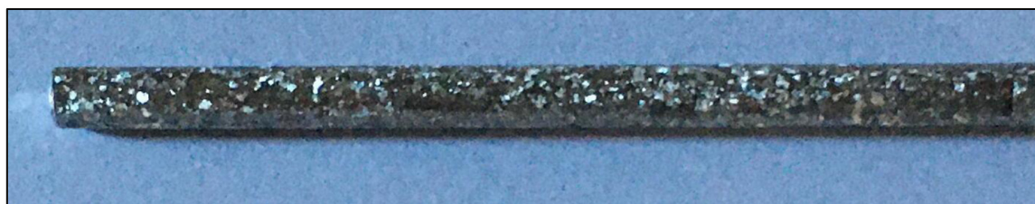
Figure 13. Palladium rod reproduced from extensive analyses of a good cathode.
