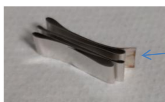
Figure 5. The sample folded to be adapted to the heater support.
