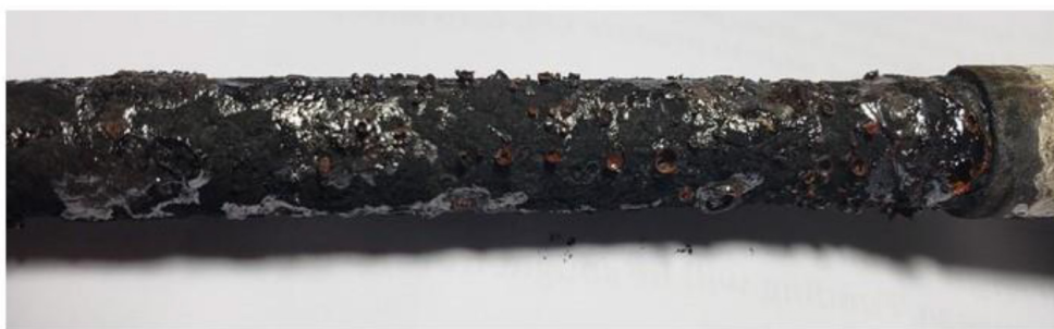
Figure 7. Photograph of the working electrode taken after the temperature test shown in figures 5 and 6.
