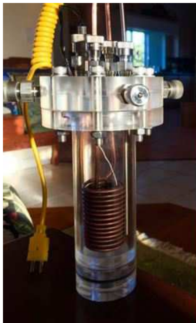
Figure 3. Shows the polycarbonate reactor with utilities entering from the top for the RF reactor passing into the cavitating Ar saturated DOD. One of the two copper coils is shown in the RF reactor where coolant water was circulated cooling the reactor operation.
