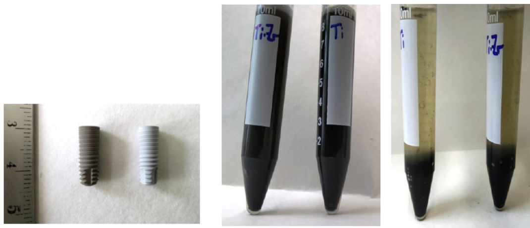
Figure 1. From Left to right. Photo of an implants made of pure titanium ( left ) and titanium with Zr protective coating ( right ) before the experiment; the appearance of tubes with implants, nutrient medium and biomass at the beginning and at the end of the experiment (in 12 days).
