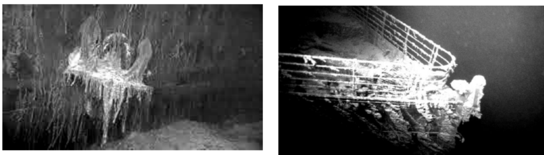
Figure 2. The growth of colonies of microorganisms on the metal parts of the Titanic [24,25].
