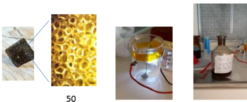
Figure 9. Nickel foam, beaker with platinum electrodes and palladium chloride solution for plating.
