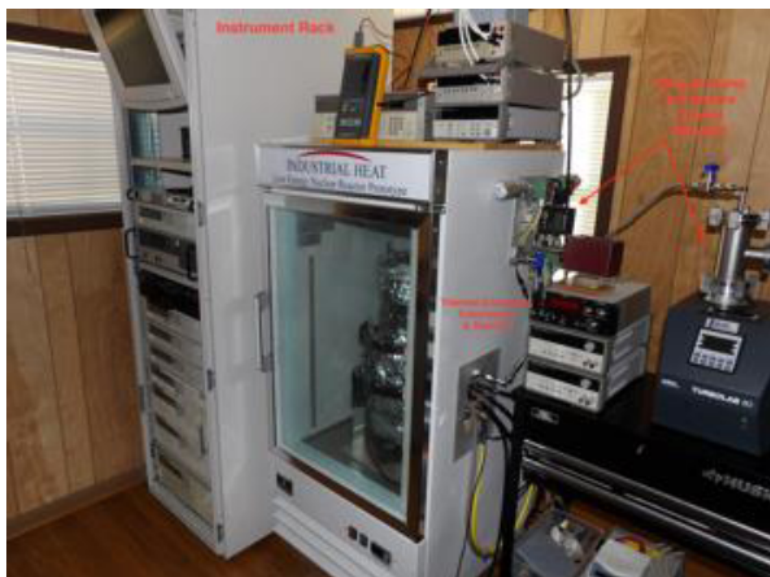
Figure 1. The instrument rack on the far left holds power supplies for system heat and fans plus the KEPCO 1000–0.2 MG power supply for the discharge. The rack also holds the lab computer that controls all instruments using LabView.
