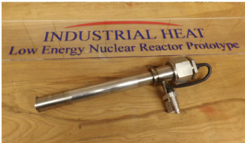
Figure 2. Figure shows the reactor used for the experiments – a 316L stainless steel tube approximately one-foot in length with an outside diameter of one-inch. Swagelok VCR connectors are used to seal the unit capable of holding vacuum to 10^{-9} Torr. High voltage DC is supplied to the reactor via a 5-kV connector obtained from MPF Products. Clamshell motor magnets (not shown) are placed around the reactor during operation and provide 230 G on the inner wall of the reactor.
