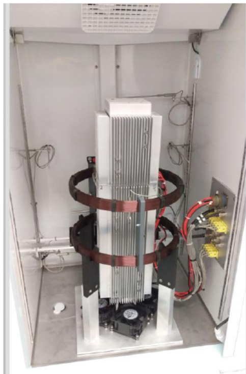
Figure 7. Figure shows the Seebeck calorimeter with the bolted lid in place, circulating fans, and data cables connected at the enclosure interface. The Helmholtz coil can be used as a listening coil for RF/acoustic signals emanating from the reactor or to apply a 40-gauss magnetic field to the reactor. Of note: the reactor produces a 3.5 kHz signal when operating and has been detected using the Helmholtz coil and verified with an Agilent spectrum analyzer.
