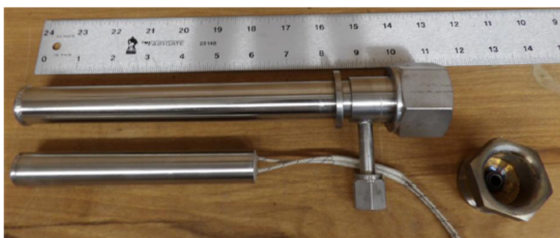
Figure 13. Figure shows the reactor and a custom fitted resistance heater used to verify that energy released in the reactor will assist in heating the thermal enclosure. In short, this is a method to simulate the release of excess power in the reactor and observe its effect on the thermal enclosure resistance heater.
