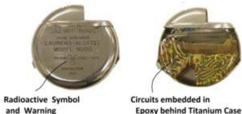
Figure 6. ^{238}\text{Pu} Cardiac pacemaker showing identification used (2.75 in. diameter, plutonium removed).
