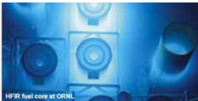
Figure 2. Irradiated neptunium at the ORNL fuel core. The blue color is Cherenkov radiation which emanates from spent fuel before it is removed from the High Flux Isotope Reactor (HFIR).
