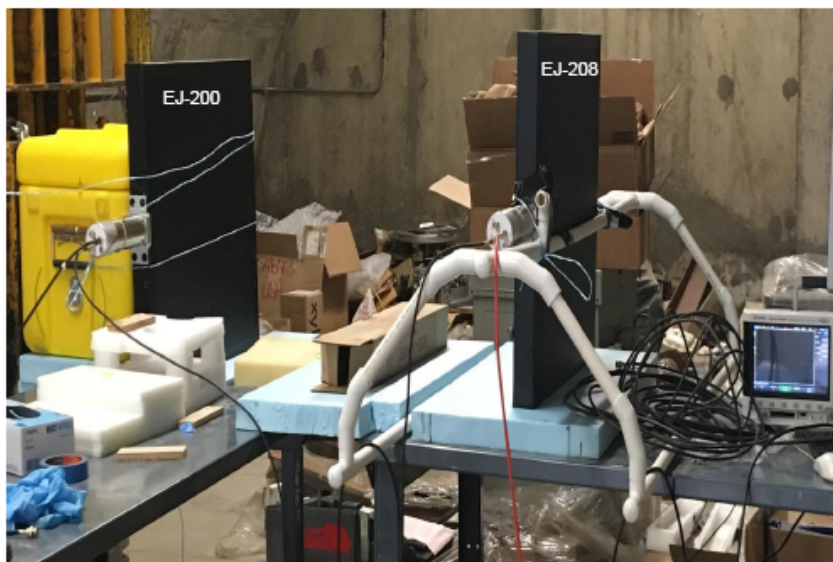
Figure 16. AmBe neutron TOF calibration in Igloo.
