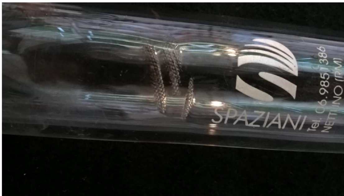
Figure 12. Picture of the borosilicate glass reactor after last experiment with air-flow calorimetry: it is clearly visible, at center, the imprint of the sheaths caused by partial melting of the internal wall due to local overheating.
