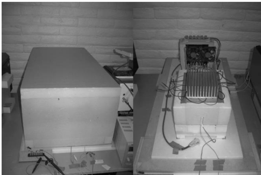
Figure 1. Coolestence calorimeter, outer box ( left ), and inner chamber with Peltier elements ( right ).
