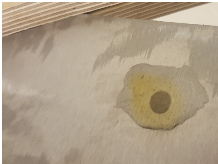
Figure 24. Photograph of the epoxy covering the HCL and Co-57 taken after the May 20 experiment.
