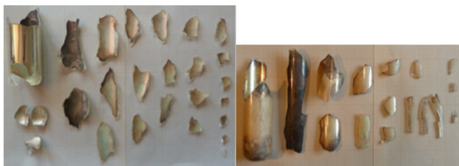
Figure 5. Left: Pieces from the outer tube. Right: Pieces from the inner tube. The cylinders visible on the left of both pictures are parts of the outer and the inner tubes and give the scale.
