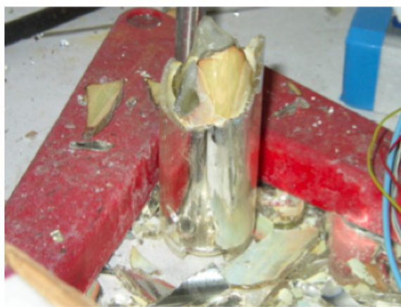
Figure 3. Photograph of the reactor after the explosion. The bottom parts remained in place, some liquid was left inside.
