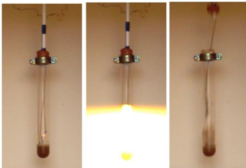
Figure 13. Deflagration ignited by a hot Constantan wire. Photographs at 33 ms intervals.
