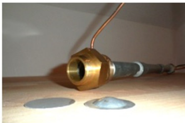
Figure 17. Picture of the reactor steel tube and of aluminum disks before and after a shot.
