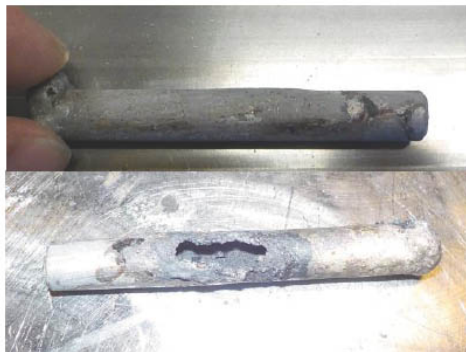
Figure 11. Post-test views of an apparently intact (slightly bloated) container and a completely breached container.
