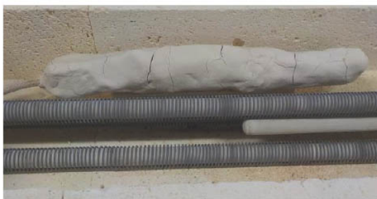
Figure 10. Photo of the container setup in this experiment. The N-type thermocouple is embedded under the porcelain encasement, and the S-type thermocouple measures the temperature between the heating spirals.
