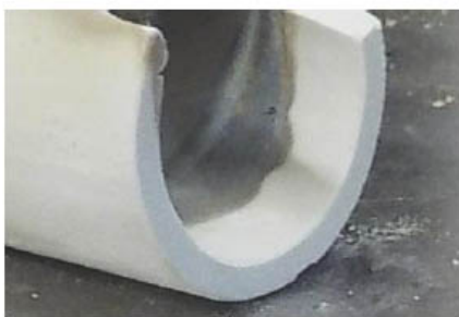
Figure 18. Post-experiment view of the downstream ceramic tube surface.
