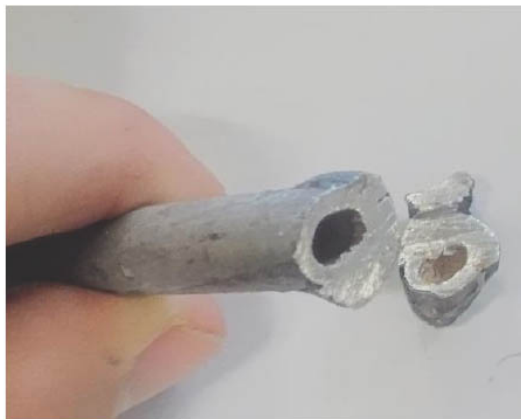
Figure 7. The cross-section view of the opened-up container, showing non-oxidized metallic surfaces along its interior.
