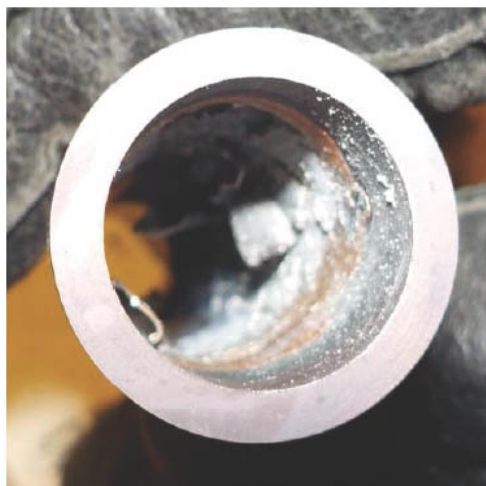
Figure 19. Post-experiment view of the reaction materials inside the TZM tube.
