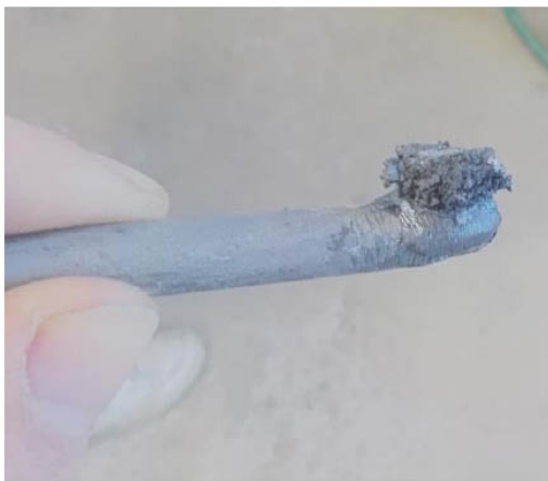
Figure 6. The container at the end of the experiment, with the view of the frozen metal geyser.
