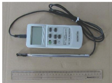
Figure 15. Air volume measurement tool for calibration.
