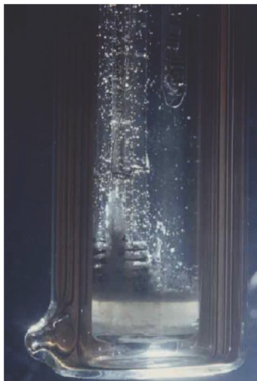
Figure 1. A photograph of an ICARUS 2 cell showing the cathode and anode and the water mixing by the hydrogen and oxygen gas bubbles.
