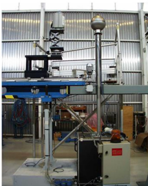
Figure 2. Experimental set-up showing a neutron dosimeter calibration. During the 18 April experiment, the neutron sources were located inside the black cubic container about 2 m from the electrolysis cell.
