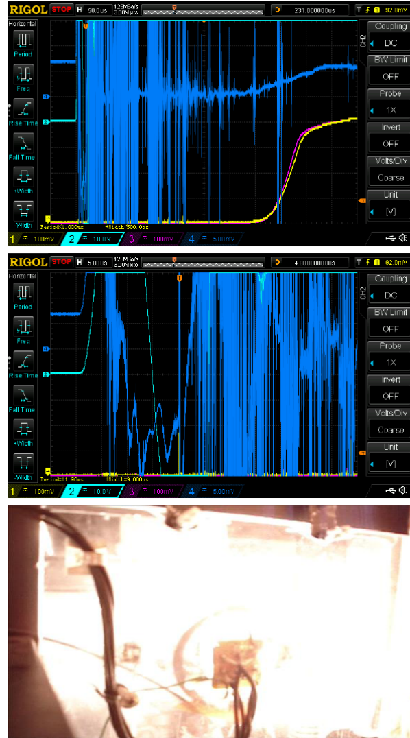
Figure 4. Oscilloscope traces for one very strong explosion, shown at 50 and 5 \mu\text{s}/\text{division} temporal resolution (use zoom 200% to view details). Blue trace is the load-cell output showing how the press applied load at 20 tons is increased above 40 tons by the explosion lasting only for 8 \mu\text{s} , followed by total fall-off and strong mechanical ringing. Turquoise trace is the output from the piezo-accelerometer, which was attached to the side of the cell until it burst. Yellow trace illustrates the response of the direct view photodiode to the debris ignition, and red trace the output from the photodiodes with UV scintillators. There is some cross-talk between the four channels because of amplifier overload. The over-exposed video camera recording of the bright explosion flash was viewed through a 12 mm thick shatterproof polycarbonate window; see Fig. 9 for mechanical layout details. The photodiodes, shown with wires attached mounted in the centre of the polycarbonate window, view through a hole but are protected from flying debris by a stainless steel mesh. Picture width corresponds to 200 mm \times 120 mm high.
