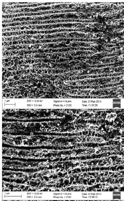
Figure 6. Images showing roughly parallel and periodic structures for 30 shots (top) and over 100 shots.
