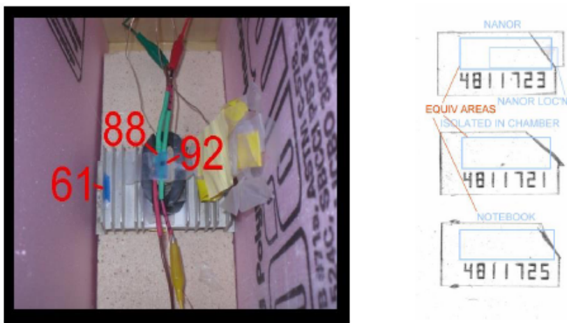
Figure 3. (a) (left) A look into the calorimeter which, for the photograph, has been stripped of thermal materials and probes to show the physical arrangement of the chips. For this image to show the location, all thermal ballast, addition thermal sensors, flow sensors, and addition insulation (both thermal and electrical) were removed. Shown are the NANOR ® (beneath chip '23, at the active site marked at #92, and the nearby chip, '21, at site #61, which was partially shielded by aluminum. The NANOR is shown below the chip, with the darkened black region (site #92) believed to be the active area at the time. The CR-39 chip was placed above the NANOR, and then thermal materials and probes replaced before the experimental run. (b) (right) The three CR-39 chips with their ID numbers, hence forth '23, '21, and '25 (left in the lab notebook).
