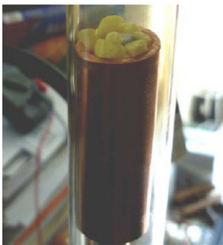
Figure 1. Sulfur and lithium atop the anode recess.
