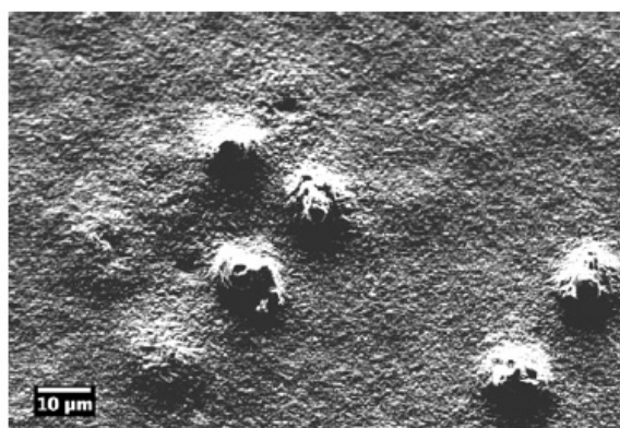
Figure 3. Surface topography of a titanium cathode after cold rolling, heating, and electrolysis in H 2 SO 4 /D 2 O.
