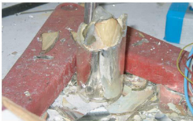
Figure 15. Broken cell after the explosion.
