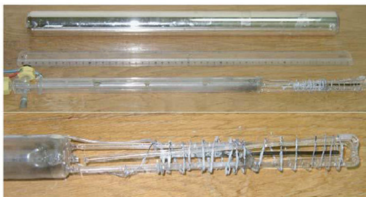
Figure 16. Interior of the cell after the explosion.
