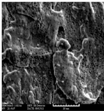
Figure 7. Surface of Ni on which Cu was deposited after heating in vacuum at 481°C.
