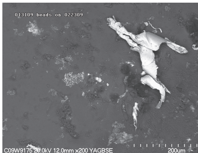
Figure 4. Spalled portion of Pd cathode after treatment with protocol. This experiment included glass beads on the cathode. Such spalling was only seen when glass beads were used.
