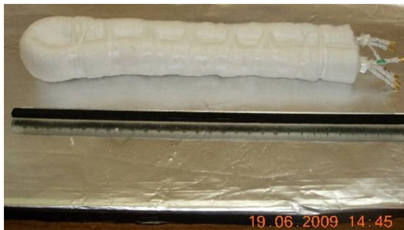
Figure 1. Wires braid inside the thermal insulation.
