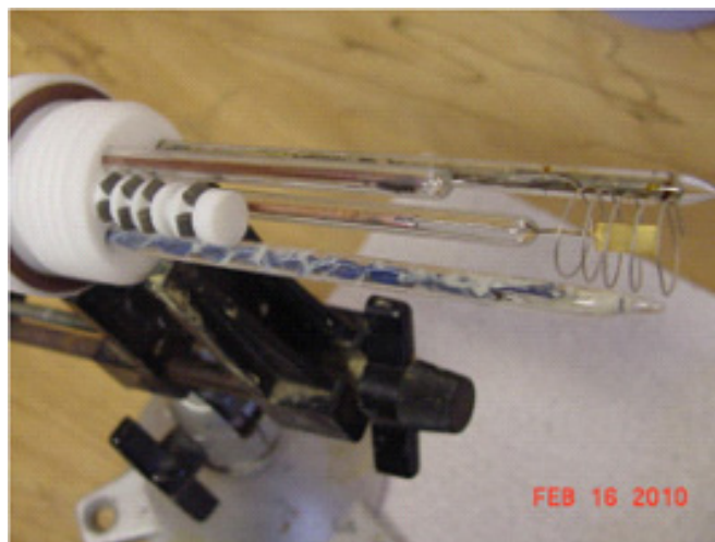
Figure 4. The electrode holders and thermistor probes are 5 mm diameter sealed glass tubes. Hook up wire is 0.5 mm platinum wire spot welded to copper wire sealed inside the glass tubes. The platinum wire is sealed against the soft glass tubing making an airtight seal. Recombiner pellets are also shown.
