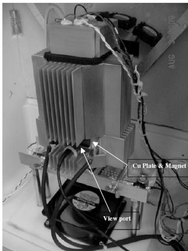
Figure 1. The Seebeck Cell Calorimeter is shown inside a temperature controlled enclosure on top of a rack with a fan to provide vigorous air stirring and a consistent airflow over the heat sinks attached to the TECs and the cell walls. Airflow temperature is controlled to \pm 0.02^\circ\text{C} , stability is \pm 0.01\text{ W} .
