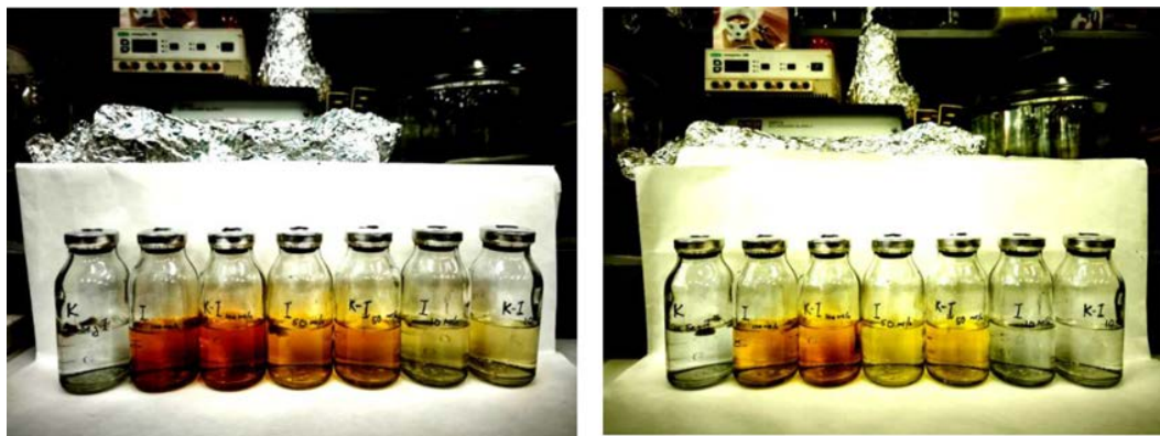
Figure 2. Two views of the system of closed bioreactors with an identical syntrophic community of mold fungi at different initial concentrations of iodine at the beginning and after the end of the experiment. Each pair of duplicate bottles contained 100, 50 and 10 mg/l of Iodine and 2% of heavy water.
