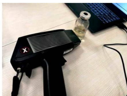
Figure 3. Detection of xenon in a bioreactor using an X-ray spectrometer SciAps X-505.
