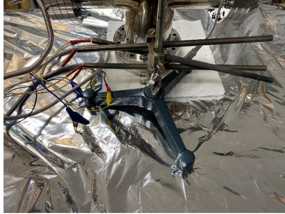
Figure 5. Three resistance heaters used to calibrate, mounted on a stand. The stand is shown here in the calorimeter chamber placed in front of a reactor. The stand is periodically moved around, and the heaters are moved up or down the pole, to confirm that moving the heat source does not affect the calorimetry.
