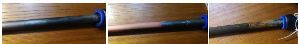
Figure 3. Titanium tube after nickel plating; titanium tube after copper plating; titanium tube after iron plating.
