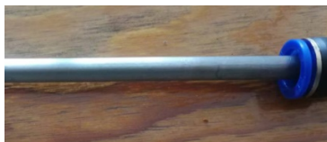
Figure 4. Titanium tube after electrolysis.
