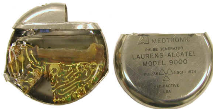
Figure 7. A plutonium powered pacemaker. The plutonium has been removed; it fit into the slot on the top left. See technical details at: https://www.ornl.gov/health-physics-museum/collection/miscellaneous/pacemaker.html .
