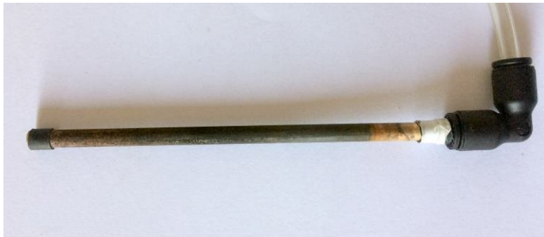
Figure 10. Oxidation appearing on the WE after exposure to air (oxidation is mainly on the left side).
